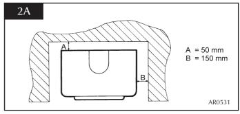
In a non-combustible recess be careful to allow enough clearance at the sides and rear of the stove to perform spillage tests and reach the controls.
